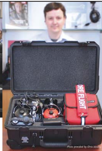
Simon Broadley, vice president of engineering for Flightcom Corporation, shows the standard wireless pushback system he and his team designed in conjunction with Southwest Airlines.
