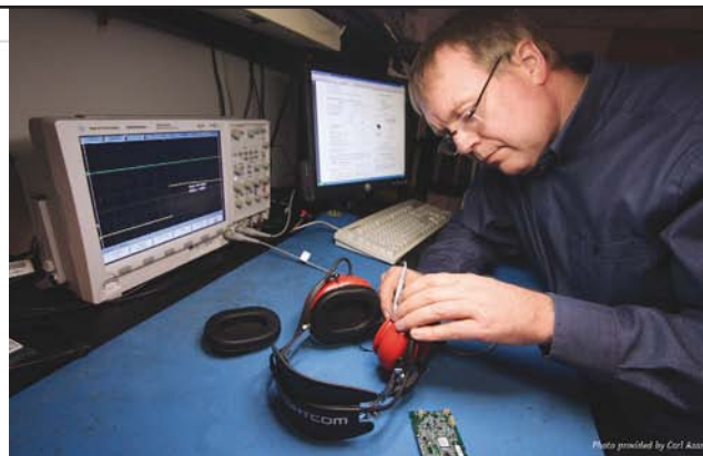
Tom Carlson, Flightcom's senior electrical engineer, adjusts the configuration on one of Flightcom's wireless ground support headsets.
