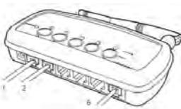
Positions 1 & 2 have radio transmit capability. All positions have intercom communications through the intercom port. Positions 3, 4, and 5 do not have radio transmit capability (any position connected via its own cable will have radio transmit capability).
