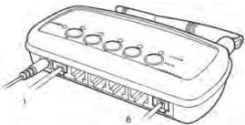
Positions 1 through 5 are radio transmit capable. PTT signal for all paired devices operate through the position 1 connection. The Intercom continues to operate through the Intercom Port.
