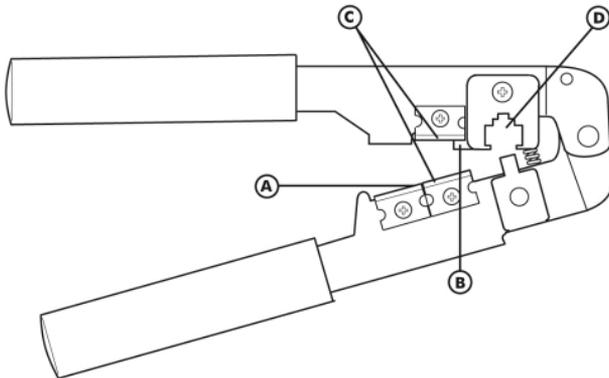
1. Using the cutter blade on the crimping tool (A), cut the flat CA Cable so the cut is clean and 90 degrees to the sides of the cable.
