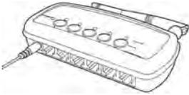
All positions communicate locally via the Base Station only. With no connection to a Digital Intercom, the Headsets will only be able to communicate with other Headsets connected to the Wireless Base Station.
