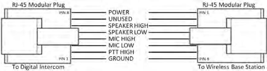
1. Connect one RJ-45 modular plug as shown above. Both the Power and Ground will be connected from the Digital Intercom to the Wireless Base Station. Any input will power the Wireless Base Station.
