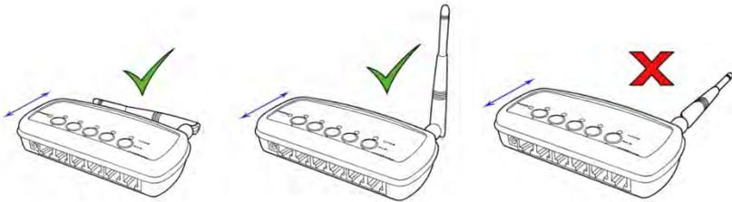
The duck antenna needs to be supported when used in a vehicle or any environment when the Wireless Base Station may be subjected to vibration.
