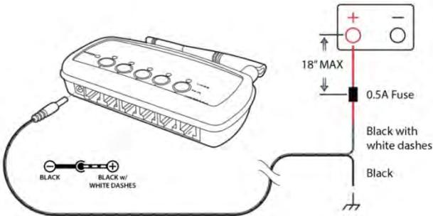
Connect the **BLACK** wire with **WHITE** dashes to +12V and the **BLACK** wire to chassis ground. Install the fuse no further than 18" from the battery.
