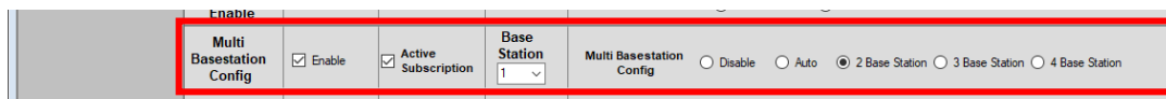
Fig. 2: The "Multi Basestation Config" row displays all options required to enable and configure the feature.
