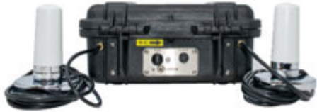
Fig. 3 (below): External coaxial connections.
