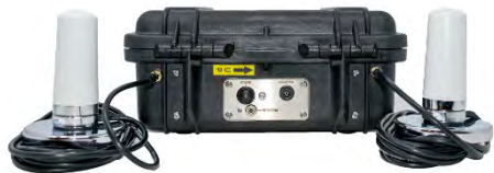
Fig. 3 (below): External coaxial connections.
