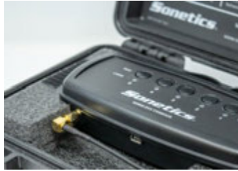
Fig. 2: Internal antenna connection.
