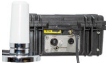
Fig. 3: External antenna connection.
